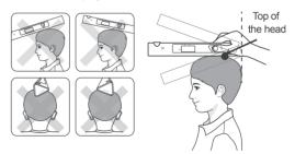
4) Press the button to measure. You can re-measure the height by pressing the button when you see horizontal bar on the screen.
